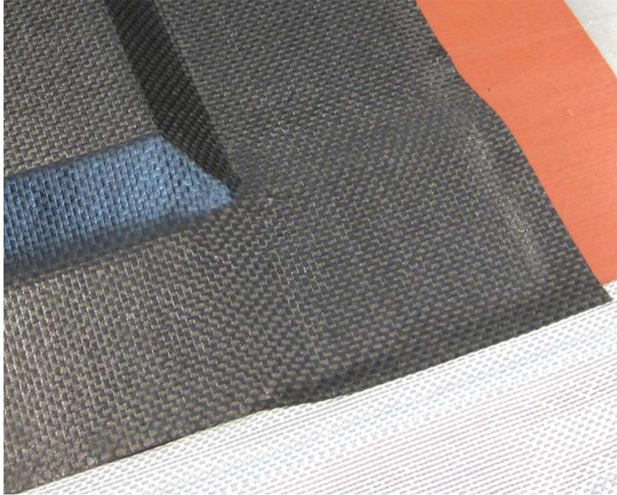
Figure 4: Stretched prepreg at corner before trimming. The two skins merge and overlap on the edge band.
