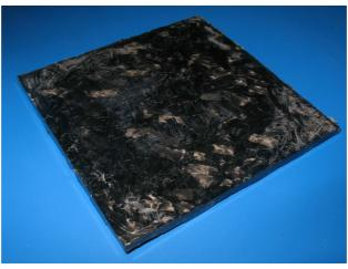
(b) Net shape flat plate obtained with this mould.
