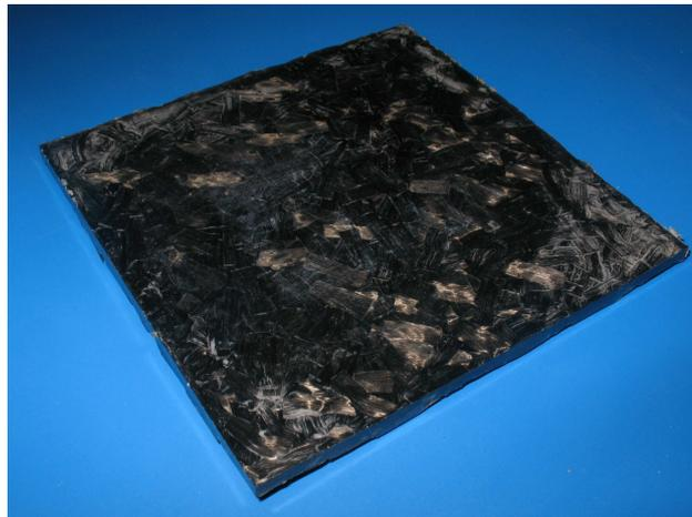
(b) Net shape flat plate obtained with this mould.
