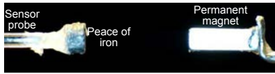
Fig. 11. Experimental setup to measure the interaction between a permanent magnet and an iron particle
