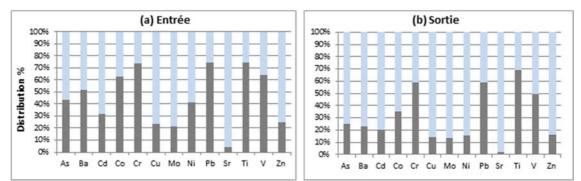
Figure 2. Distribution of metals between the dissolved and particulate phases of the dry basin: (a) inlet (b) outlet
