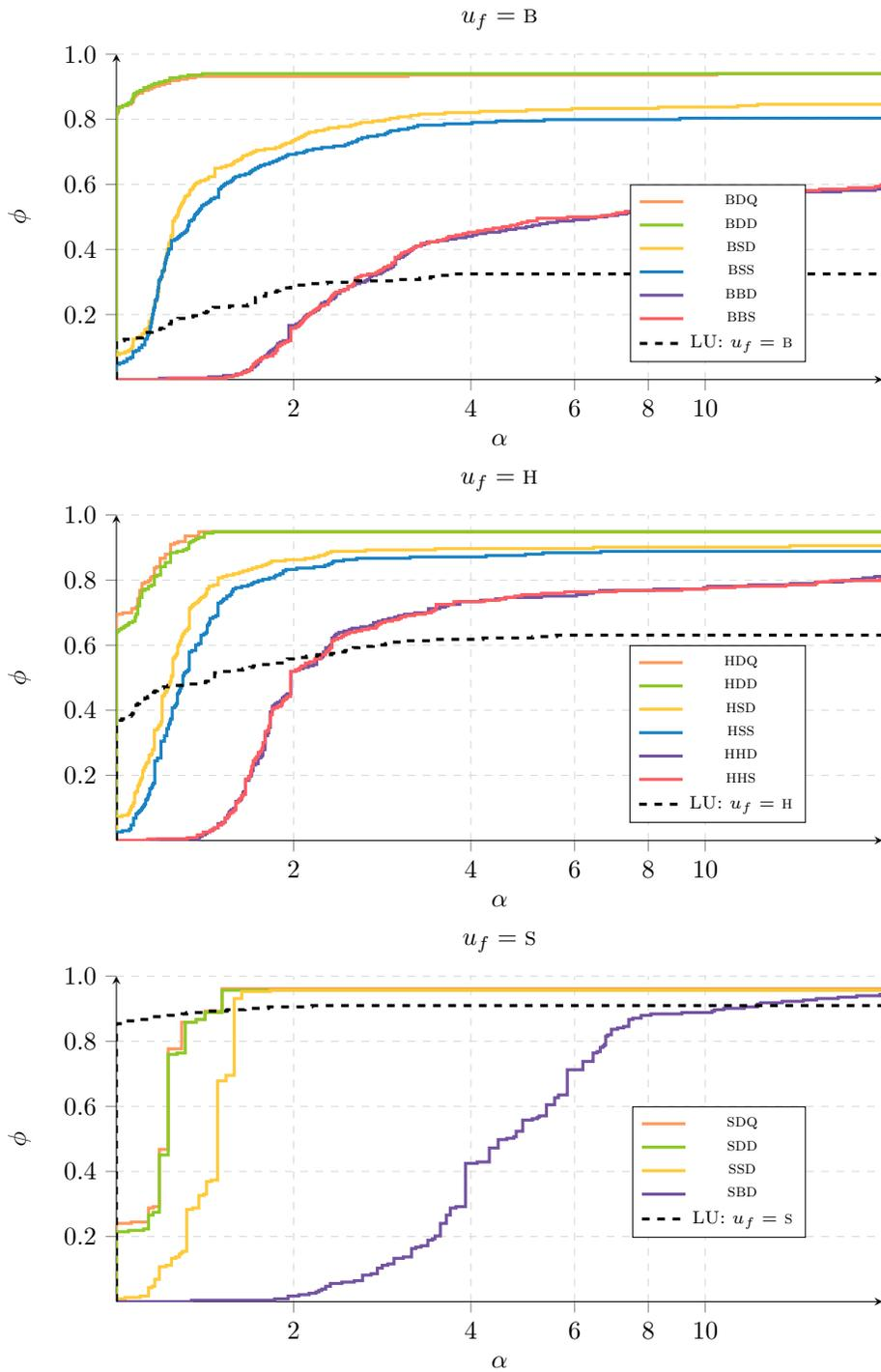
FIG. 4.3. Performance profile of LU-IR3 and GMRES-IR5 variants (with  $u_f$ ,  $u_g$ ,  $u_p$  as specified in the legend) on 230 SuiteSparse matrices.  $\phi$  (y-axis) indicates the percentage of matrices for which a given variant requires less than  $\alpha$  (x-axis) times the number of LU solves required by the best variant.
