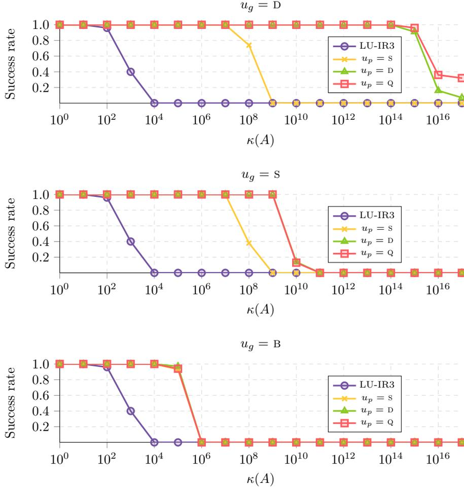
FIG. 4.1. Proportion of matrices for which LU-IR3 and GMRES-IR5 with varying  $u_p$  and  $u_g$  converged to double precision forward error as a function of  $\kappa(A)$ . For all variants,  $u_f = B$ ,  $u = D$ , and  $u_r = Q$ .
