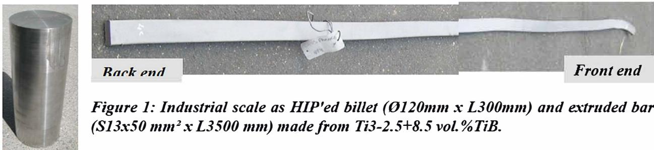
*Figure 1: Industrial scale as HIP'ed billet ( $\text{Ø}120\text{mm} \times L300\text{mm}$ ) and extruded bar ( $S13 \times 50\ \text{mm}^2 \times L3500\ \text{mm}$ ) made from Ti3-2.5+8.5 vol.%TiB.*
