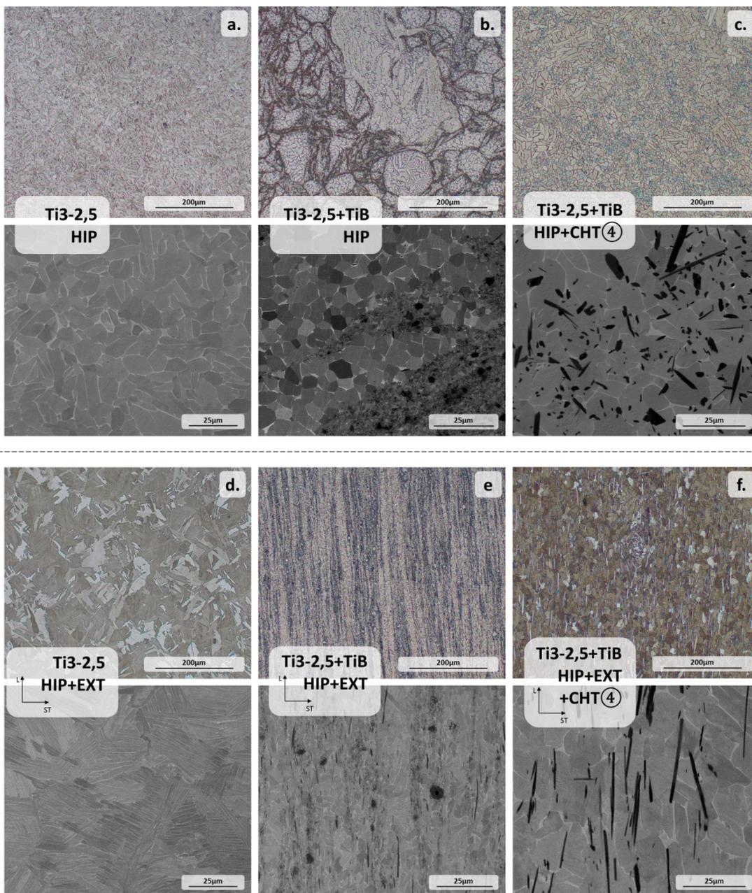
**Figure 2: OM micrographs (on top) and SEM micrographs (on the bottom) of the various produced specimens described in Table 2.**
