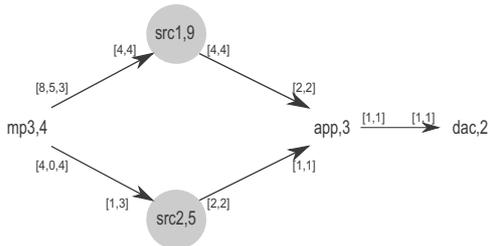
Figure 1. CSDF graph of the MP3 application
