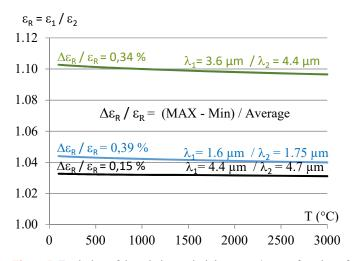
Figure 7: Evolution of the relative emissivity  $\mathcal{E}_R = \mathcal{E}_1 / \mathcal{E}_2$  as a function of temperature for different choices of wavelengths  $\lambda_1$  and  $\lambda_2$  according to the extended Hagen-Ruben analytical model [25].
