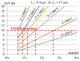
Figure 11: Evolution of the temperature precision  $\Delta T/T$  as a function of the relative emissivity precision  $\Delta \varepsilon_{R}/\varepsilon_{R}$  for different surface temperatures. The ITER requirement is  $\Delta T/T < 10\%$ .
