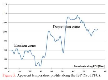
For the ITER thermography this is not acceptable since the requirements indicates  $\Delta T/T < 10\%$  over the entire temperature range from 200 °C to 3 600 °C.
