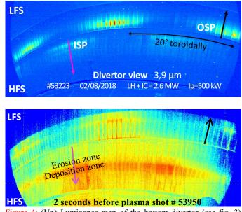
Figure 4: (Up) Luminance map of the bottom divertor (see fig. 3) during plasma operation. (Down) Luminance map of the bottom divertor 2 seconds prior of shot #53950. The luminances are far from being homogeneous, underlying the non-uniform emissivity.
