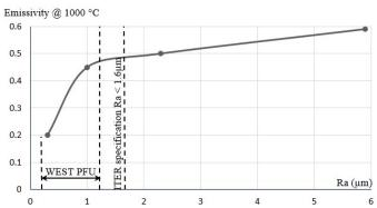
Figure 1: Emissivity evolution at 1000 °C for roughness between  $Ra = 0.3 \ \mu m$  and  $6 \ \mu m$ .
