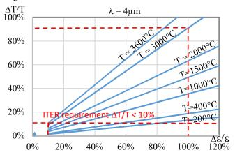
Figure 6: Monocolor temperature precision  $\Delta T/T$  at 4µm as a function of the emissivity precision  $\Delta \epsilon/\epsilon$  for different temperatures. Note that the ITER requirement is  $\Delta T/T < 10\%$  over the temperature span from 200°C to 3600°C.
