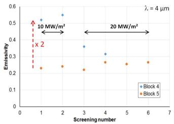
Figure 2: Emissivity variation with screening number at 10 and 20 MW/m<sup>2</sup> for 2 adjacent monoblocks located on the same actively cooled ITER-like plasma facing unit mockup [26].
