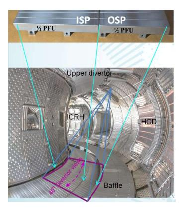
Figure 3: (Up) picture of the 2 parts of semi-inertial plasma facing unit made of graphite covered with a layer of 10  $\mu$ m of tungsten. (Down) Tangential view of WEST equipped with tungsten covered graphite tiles.
