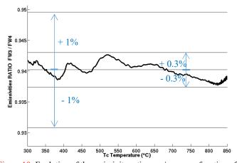
Figure 10: Evolution of the emissivity ratio  $\epsilon_{FW3}/\epsilon_{FW4}$  as a function of the Tc temperature. The fixed value taken at 350 °C for the emissivity ratio is 0.9402 for the bicolor temperature estimation.
