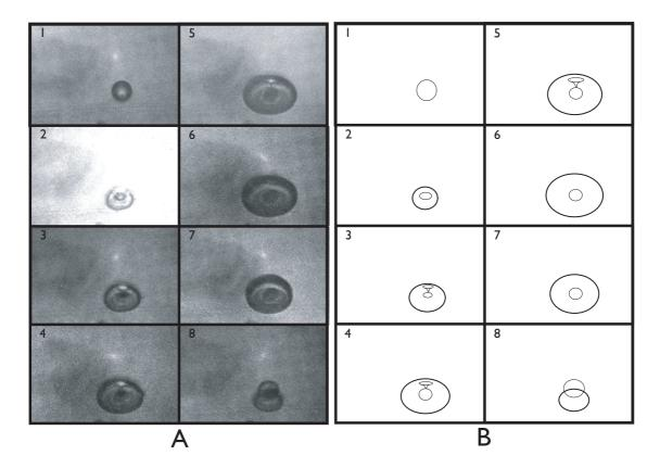
**FIGURE 1.** Gas release from a lipid-shelled microbubble (A) and a schematic representation thereof (B). The frames were captured at 3 million frames per second. Frame 1 has been taken prior to ultrasound arrival. Frames 2–8 cover one full ultrasonic cycle. Each frame corresponds to a  $88 \times 58 \,\mu m^2$  area. The images were captured at the Department of Experimental Echocardiography, Thoraxcentre, Erasmus MC, Rotterdam, The Netherlands.
