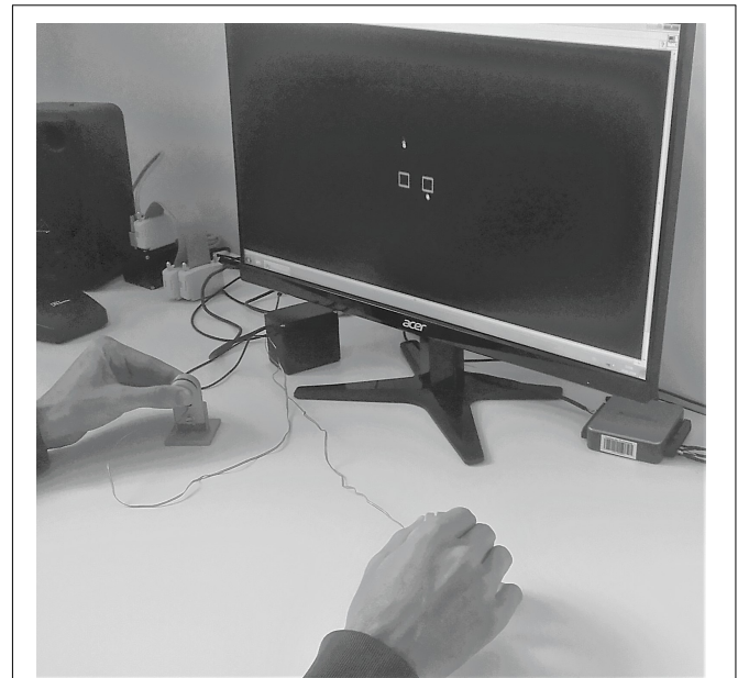
FIGURE 3 | Participant's point of view during execution of the experimental procedure. The participant applies force to the two force transducers using a pinch grip with thumbs and index fingers of both hands. Feedback of the magnitude of his/her applied force is given by the yellow dots on the screen. The square boxes indicate the reference force levels.
