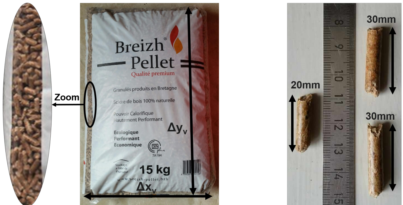
Figure 3. Bag of wood pellets used to simulate a volume and picture of pellet items.
