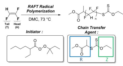
Figure 1. Scheme of the RAFT polymerization of TrFE, using tert-amyl peroxy-2-ethylhexanoate as initiator, O-ethyl-S-(1-methoxycarbonylethyl)dithiocarbonate as CTA and dimethylcarbonate as solvent.
