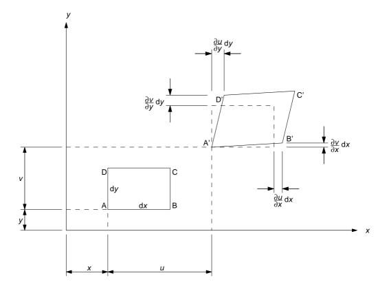
Figure 8.1: Stressing an element.
