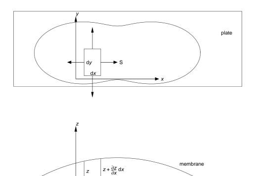
Figure 18.1: Edge-supported membrane spanning a hole in a plate.
