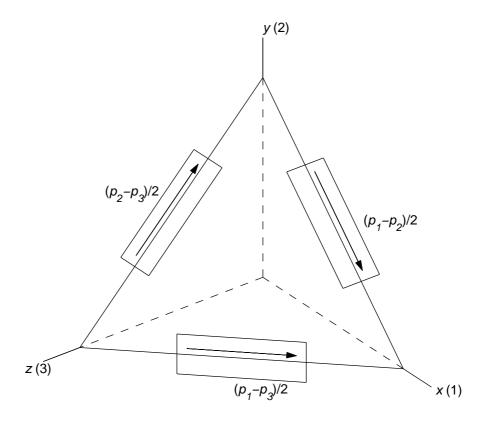
Figure 5.2: Planes of maximum shear stresses.
