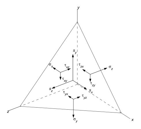
Figure 2.2: State of stress on a tetrahedron.
