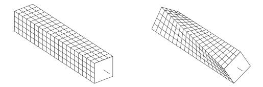
Figure 17.1: Rectangular bar (left) subjected to warping (right).
