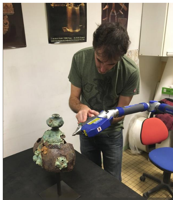
Figure 15 – 3D acquisition by lasergrammetry of a Gallic helmet found on the Tintignac-Naves archaeological site. The laser scanner is a Faro scan arm (Archeovision production - 2018)
