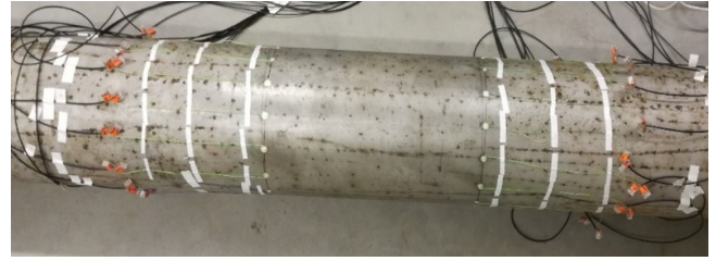
Fig. 2: Experimental setup. Picture of the pipe with the bounded piezoelectric transducers.
