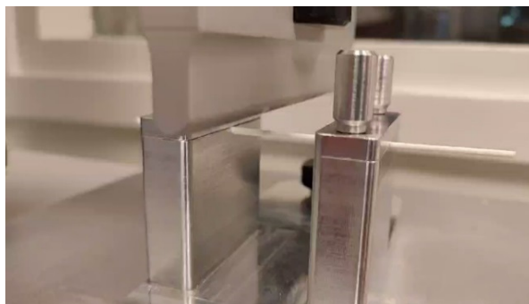
Figure 1. 3 points bending setup with attached filament.
