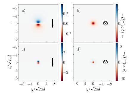
Figure 5: Dimensionless deformation fields at the free surface of two soft substrates, for a sphere placed at a unit distance D = 1 and for two modes of motion. In a) and b), the substrate's mechanical response follows the Winkler foundation (see Eq. (56)). In c) and d), the substrate's mechanical response is the one of a thin incompressible layer (see Eq. (67)).
