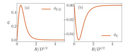
Figure 4: Scaling functions for  $P_1^{(1)}$  (see Eq. (28)), obtained from numerical integration of Eq. (26), with the boundary conditions  $P_1^{(1)}(R =$ (0,T) = 0 and  $P_1^{(1)}(R \to \infty, T) = 0$ .
