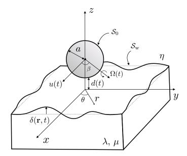
Figure 1: Schematic of the system. A rigid sphere of surface  $S_0$  is freely moving in a viscous fluid, near a soft wall of surface  $S_w$  in the flat undeformed state. The lubrication pressure field deforms the latter which induces an elastohydrodynamic coupling, with forces and torque exerted on the sphere. Note that the surface deformation is magnified for clarity, but that we restrict the analysis to the  $\delta \ll d$  case.
