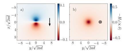
Figure 2: Dimensionless deformation fields at the free surface of the soft substrate, for a sphere placed at a unit distance D=1 and for two modes of motion: a) the sphere velocity is directed tangentially to the substrate, along the x-axis (see black arrow), and is fixed to a unit value U=1; b) the sphere is approaching the substrate normally (see black cross) with a unit velocity  $\dot{D}=-1$ .
