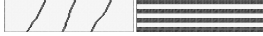
Fig. 1 Testcase 1 – partition ( N = 4 ) and distribution of E ( 10^8 if white and 10^3 if dark)
