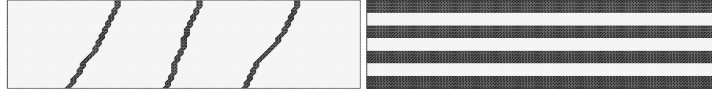
Fig. 1 Testcase 1 – partition into N = 4 subdomains and distribution of E ( 10^8 in white layers and 10^3 in dark layers)
