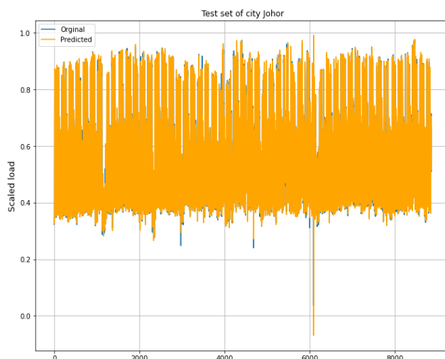
FIGURE 31. Actual and predicted load consumption from LSTM, Malaysian data.
