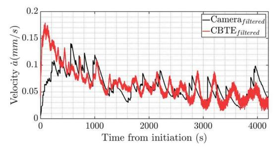
Figure 10: Crack velocity time history using the CBTE analysis and a camera for the monitoring of the crack tip position, for a test performed with  $\dot{\delta}=0.5$ mm/min
