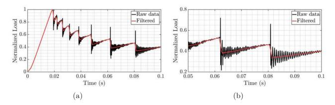
Figure 5: (a) Load-Displacement curve for  $\dot{\delta} = 5000 mm/min$ . (b) Effect of the mean local filter on the signal
