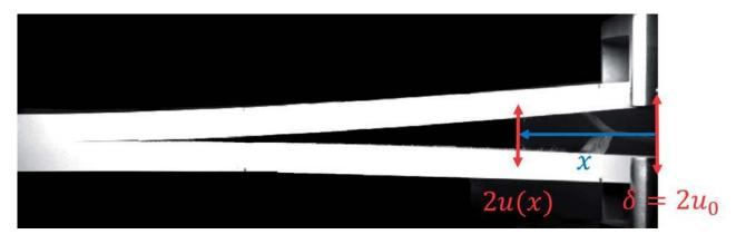
Figure 1: Double Cantilever Beam test
