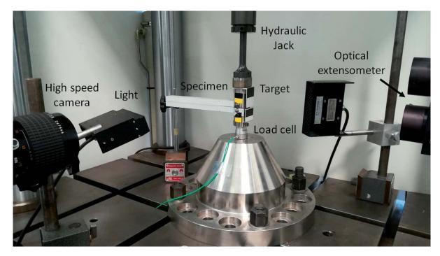
Figure 3: Experimental set up
