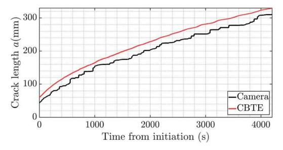
Figure 8: Comparison of the measured crack length using the extended CBTE and the camera monitoring for a test performed with  $\dot{\delta}=0.5$ mm/min
