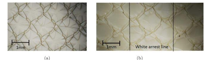
Figure 7: Post mortem microscopic view of the crack surface for (a) steady-state propagation and (b) "stick-slip" mechanism
