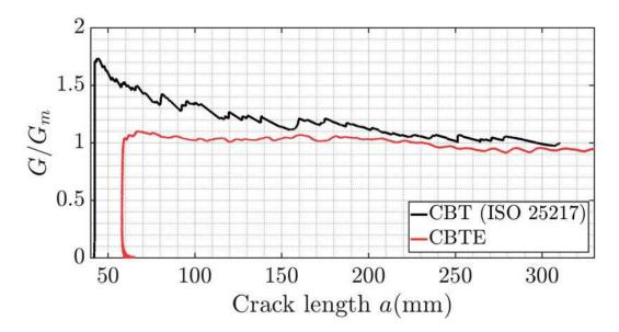
Figure 9: Comparison of the energy release rate using the extended CBTE and the standard CBT for a test performed with  $\dot{\delta}=0.5$ mm/min
