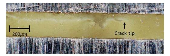
Figure 2: Crack tip observation after the precracking operation in the joint using a microscope Hirox RH-2000  $\,$
