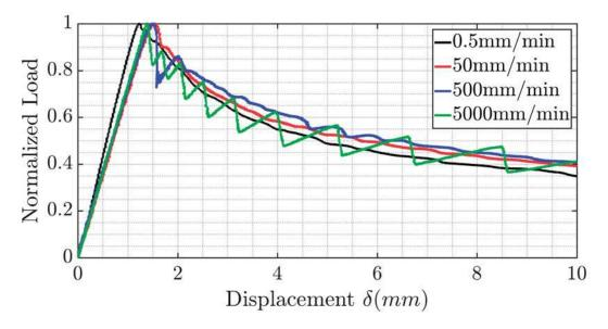
Figure 4: Load-Displacement curves for different loading rates
