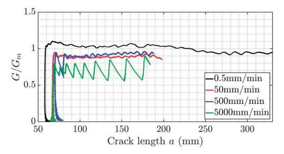
Figure 11: Normalized R-curve for different loading rates : Energy release rate using the CBTE analysis
