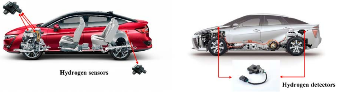
Fig. 2. Hydrogen detectors/sensors locations in the commercialized FCEV: left-side: Honda Clarity FCEV [6]; right-side: Toyota Mirai [7].
