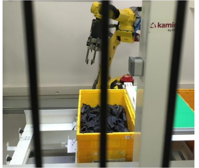
Fig. 1. Real robotics setup with an industrial Fanuc robot for a grasping task from homogeneous highly cluttered heap of elbowed rubber tubes.
