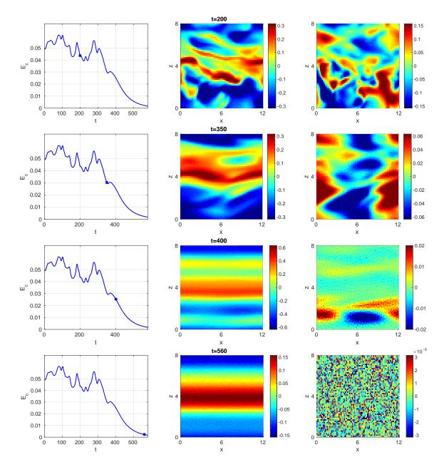
Figure 16: Collapse of turbulence in a very small system of size  $L_x \times L_z = 12 \times 8$ . Left column: time series of kinetic energy with dot indicating the instant in the simulation. middle column, colour levels of streamwise velocity in the horizontal midplane. Right column: colour levels of spanwise velocity in the horizontal midplane.
