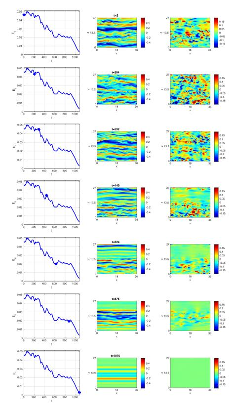
Figure 12: Following a collapse trajectory in a domain of size  $L_x \times L_z = 36 \times 27$ , R = 377. The left panels show a time series of kinetic energy, with the dot indicating the instant at which the colour levels of streamwise velocity in the y = 0 plane (middle panels) and spanwise velocity (right panels) at corresponding times in the y = 0 plane are shown. 22
