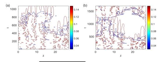
Figure 14: Contours of  $\sqrt{\int_{x=0}^{36} u_z^2 dx - \left(\int_{x=0}^{36} u_z dx\right)^2} = 0.03$  and  $\sqrt{\int_{x=0}^{36} u_x^2 dx} = 0.15$  as a function of z and t for (a) the collapse trajectory of figure 12 and (b) the non reactive trajectory of figure 13.
