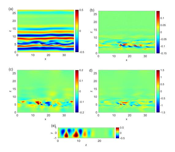
Figure 11: Colour levels of the streamwise (a), wall normal (b) and spanwise (c) components of the velocity field, in the y = 0,  $\vec{e_x} \times \vec{e_z}$  plane for the last stage at the last branching step in an AMS computation of collapse trajectories at R = 377 in a domain of size  $L_x \times L_z = 36 \times$ , along with (d) the streamwise vorticity. (e) Colour levels of streamwise averaged streamwise velocity as a function of y and z for the same state.
