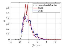
Figure 7: Normalised distribution of duration of collapse trajectories sampled by AMS ( $\simeq 1600$  samples), by DNS ( $\simeq 189$  samples) and compared to a normalised Gumbel distribution, in a system of size  $L_x \times L_z = 24 \times 18$  at Reynolds number R = 370.
