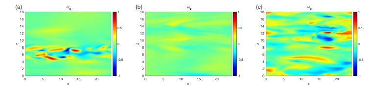
Figure 6: Streamwise vorticity in the midplane y = 0 in the system of size  $L_x \times L_z = 24 \times 18$  for last states at the last branching stage of several AMS computations. (a) Run estimating  $\hat{\alpha} = 0.045$ ,  $\hat{T} = 1.5 \cdot 10^4$ , (b) run estimating  $\hat{\alpha} = 0.086$ ,  $\hat{T} = 1.1 \cdot 10^4$ , (c) run estimating  $\hat{\alpha} = 0.022$ ,  $\hat{T} = 3.7 \cdot 10^4$ .
