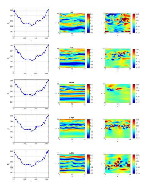
Figure 5: Time series of the kinetic energy (left panels) with a dot indicating the point in time of each line (t = 2, t = 74, t = 200, t = 400, t = 600), alongside colour levels of the streamwise velocity (central panels) and spanwise velocity (right panels) in the midplane y = 0 during a non reactive trajectory (hole opening then closing), at corresponding times, in a domain of size  $L_x \times L_z = 24 \times 18$  computed by AMS.
