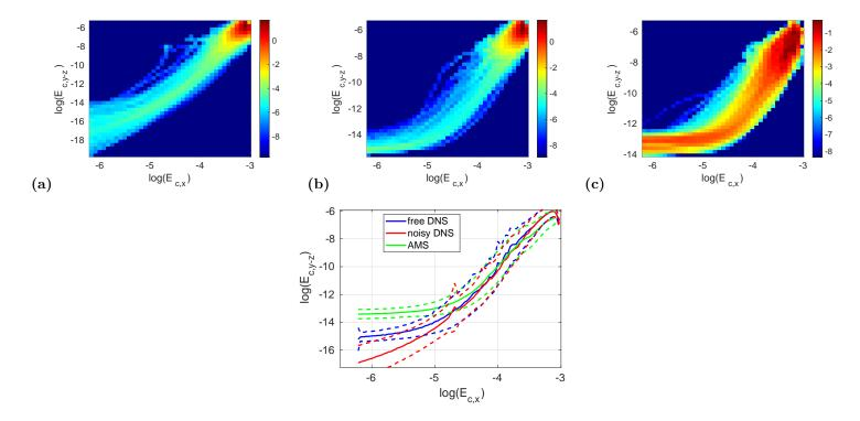
Figure 8: Probability density functions in the  $(E_{c,x}, E_{c,y-z})$  plane, conditioned on being in a collapse trajectory, for (a) Trajectories from free DNS, (b) trajectories from noisy DNS, (c) 1138 trajectories from AMS. (d) Conditional Average trajectories and their variances.
