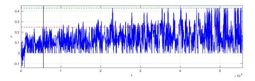
Figure 15: Time series of  $\Phi$  during an AMS calculation with the  $24 \times 16$  system leading to extinction (the laminar state corresponds to  $\phi \ge 1$ ). The black line indicates the end of the stage 0 of AMS and the red line the maximal  $\phi = 0.248 \pm 0.001$  reached during this stage ("contained in the initial conditions"). The green line indicate the maximum  $\phi = 0.430 \pm 0.001$  reached during the whole AMS calculation.
