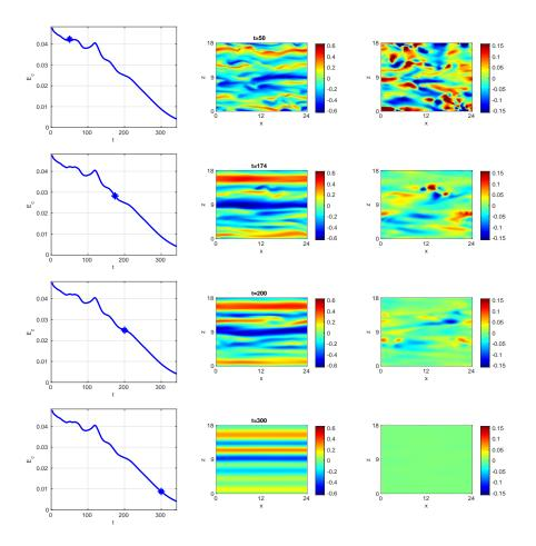
Figure 4: Time series of the kinetic energy (left panels) with a dot indicating the point in time of each line (t = 50, t = 174, t = 200, t = 400), alongside colour levels of the streamwise velocity (central panels) and spanwise velocity (right panels), at corresponding times, in the midplane y = 0 during a collapse trajectory in a domain of size  $L_x \times L_z = 24 \times 18$  computed by AMS.
