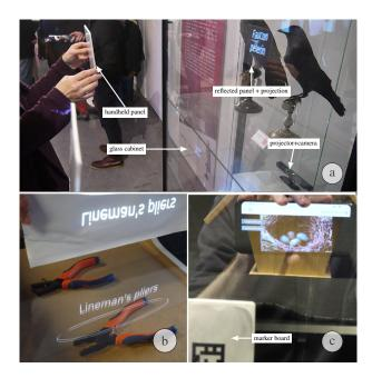
Figure 2: Implementation of Revealable Volume Display: (a) Projector + depth camera implementation with a visitor revealing the name of an exhibited bird, (b) Horizontal configuration with objects below the glass panel and text annotations revealed using a sheet of paper, (c) Mobile implementation of RVD
