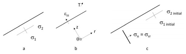
Figure 4 : Mechanical and thermo mechanical stresses: a - Mechanical stresses; b - Stresses / strain linked to thermal variations; c - Fracture perpendicular to the free surface submitted to tension and initial stresses
