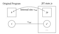
(b) In the external simulation relation,  $s \approx_{ext} js$  iff 1) there exists an (internal) backward simulation between jp and p using relation  $\approx_{int}$  and 2) s is matched with s' using  $\approx_{int}$ .
