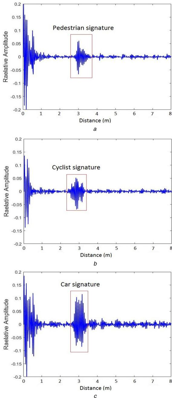
**Fig. 13** Signatures of the three different targets
