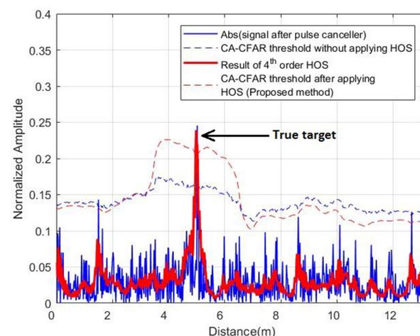
**Fig. 9** Comparison of the CA-CFAR performance run directly on the signal without time-delay estimation and with time-delay estimation (HOS),  $P_{fa} = 10^{-5}$ ,  $M = 150$  and  $N = 2$ . A real target presents 5 m away from the radar
