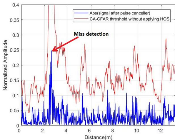
**Fig. 7** Miss detection of CA-CFAR,  $P_{fa} = 10^{-5}$ ,  $M = 20$  and  $N = 2$
