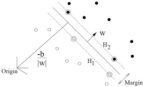
**Fig. 1** Illustration of support vectors, hyperplane and margin
