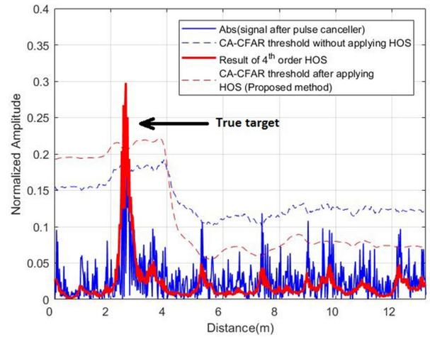
**Fig. 10** Comparison of the CA-CFAR performance run directly on the signal without time-delay estimation and with time-delay estimation (HOS),  $P_{fa} = 10^{-5}$ ,  $M = 150$ , and  $N = 2$ . A real target presents 2.5 m away from the radar
