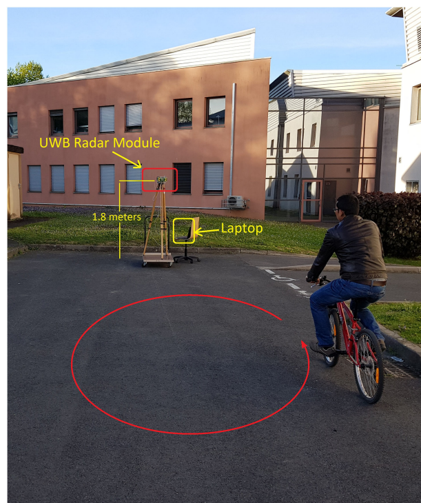
Fig. 2 Radar setup and an example of an experiment where a cyclist moved in front of the radar
