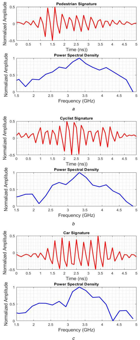
**Fig. 14** Normalised signatures of the three different targets followed by their power spectral densities. As can be seen, the figure shows that the different natures of the radar target yielded different radar signatures
