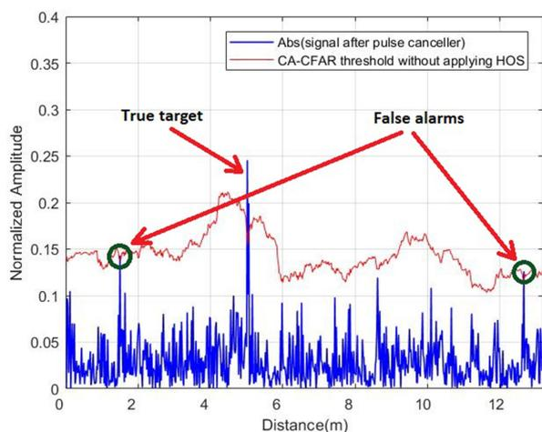
**Fig. 6** CA-CFAR detects false alarms,  $P_{fa} = 10^{-5}$ ,  $M = 80$  and  $N = 2$
