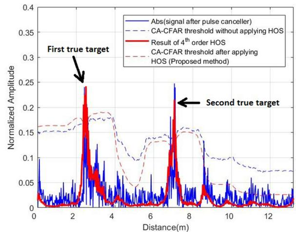
**Fig. 11** Comparison of the CA-CFAR performance run directly on the signal without time-delay estimation and with time-delay estimation (HOS),  $P_{fa} = 10^{-5}$ ,  $M = 150$  and  $N = 2$ . Two real targets present at 2.5 and 7 m away from the radar
