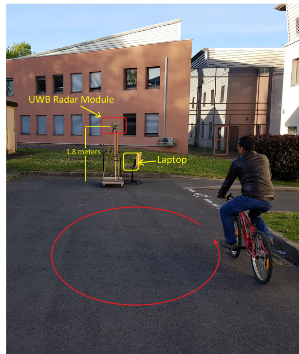
Fig. 2 Radar setup and an example of an experiment where a cyclist moved in front of the radar
