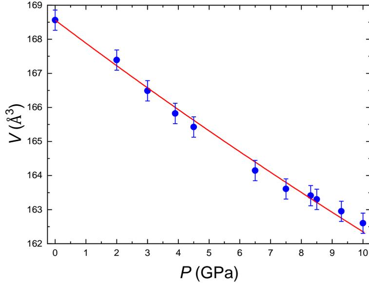
**Figure 12.** Unit-cell volume of  $\text{Hf}_{0.75}\text{Ta}_{0.25}\text{Fe}_2$  as a function of applied pressure. The continuous red line represents the third-order Birch-Murnaghan fit for the data.
