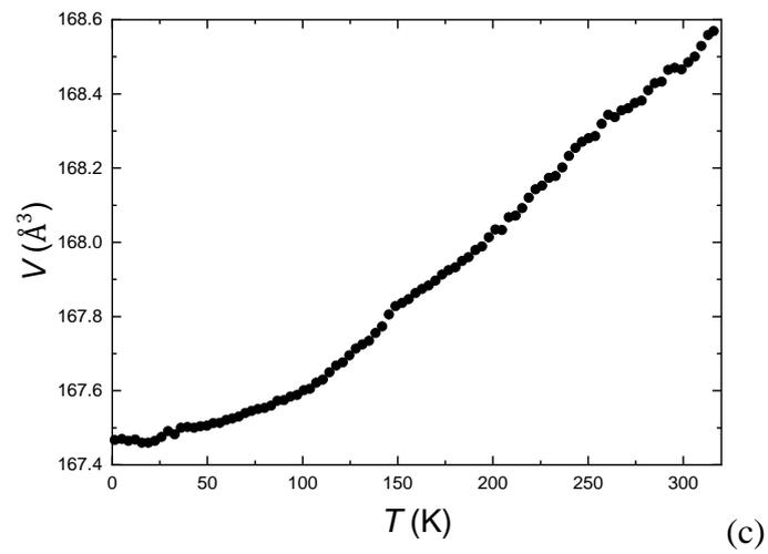
**Figure 6.** Thermal dependence of the lattice parameters  $a$  and  $c$  (a),  $c/a$  ratio (b), and unit-cell volume (c) obtained from Rietveld refinement of NPD data measured upon heating for  $\text{Hf}_{0.75}\text{Ta}_{0.25}\text{Fe}_2$ .
