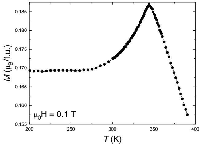
**Figure 1.** Temperature dependence of the magnetization for  $\text{Hf}_{0.75}\text{Ta}_{0.25}\text{Fe}_2$ .
