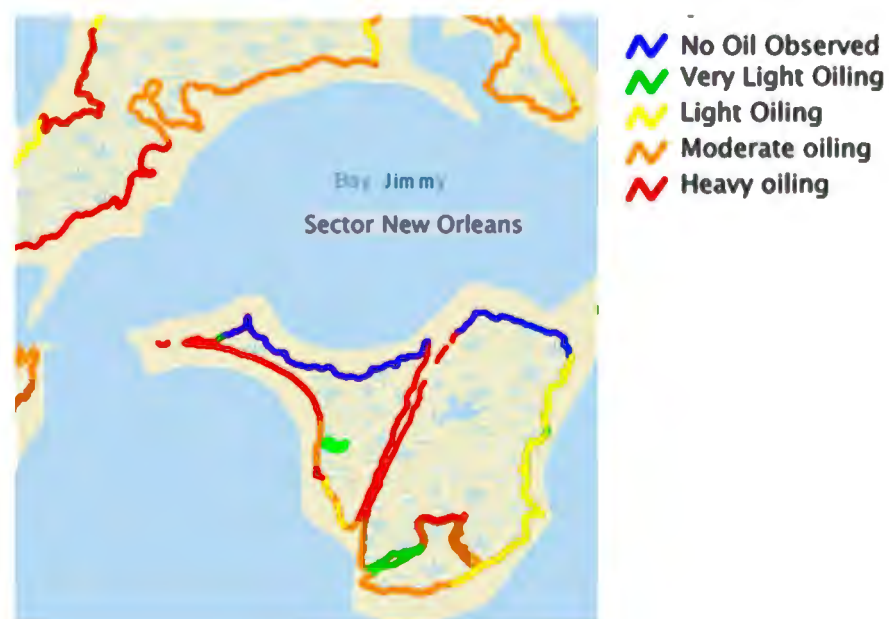
Figure 13. Environmental Response Management Application (ERMA), 17 September 2010—SCAT (Shoreline Cleanup and Assessment Technique) oiling ground observations [45].
