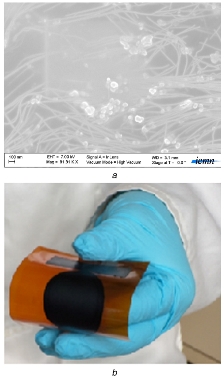
Fig. 1 Formation PANI/MWCNTs nanocomposites (a) SEM images of nanocomposite PANI/MWCNTs, (b) Photograph of the fabricated film
