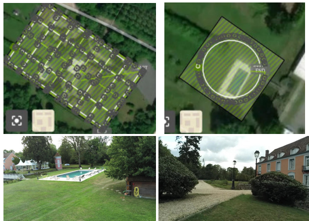
Figure 7. Video acquisition process of the Manoir dataset. Top: grid and orbit flight plan used for photogrammetry. Bottom: Video samples from the Anafi drone, 4k (left) and 720p (right)
