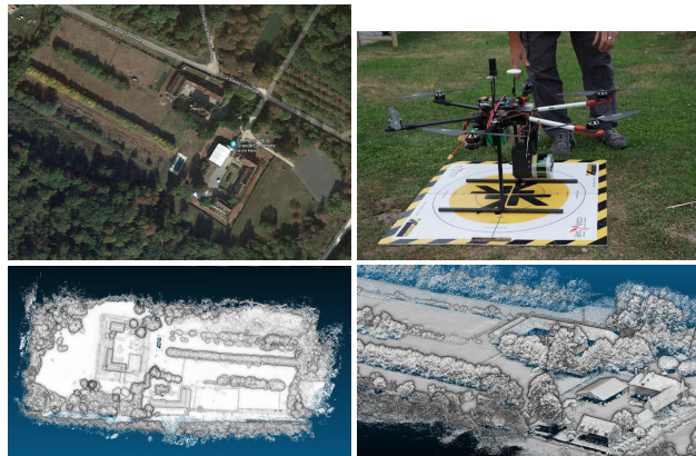
Figure 6. 3D Mapping process of the Manoir dataset. Top: map of the scanned area and scan device used for mapping. Bottom: two views of the resulting point cloud.
