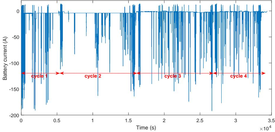
Figure 7: Driving cycles used for parameter identification
