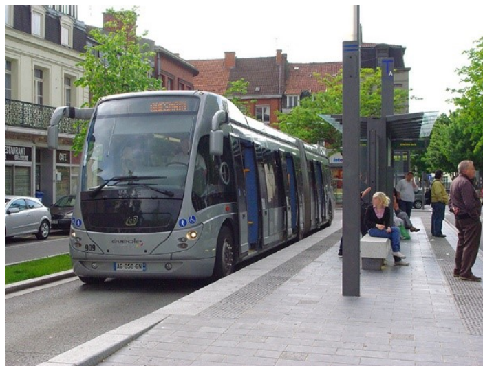
Figure 15 - Phileas of Douai: vehicle has access doors on both sides, June 12, 2010.
