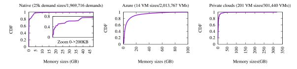
Figure 2: CDF of memory allocation sizes in different datacenter types.
