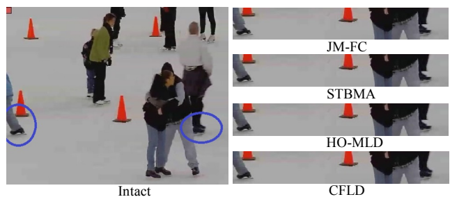
Fig. 13: Visual comparison of a reconstructed frame with H.264 Ice sequence at QP=37 by different methods. One bit was flipped in frame 45, slice 22 and bit 381. The packet contains 472 bits. The proposed checksum provides 11 candidates. The first valid candidate which satisfied the two mentioned conditions is picked as CFLD output and the packet was perfectly corrected. The PSNR and SSIM values of each approach are as follows, respectively: Intact (36.49 dB, 0.9681), JM-FC (34.12 dB, 0.9649), STBMA (34.37 dB, 0.9659), HO-MLD (34.39 dB, 0.966) and CFLD (36.49 dB, 0.9681).
