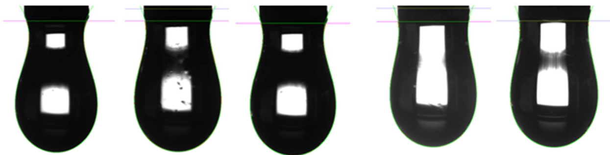
Figure 6: Pendant drop profiles at 200°C for zPE, rPE, mPE, ziPP and miPP (from left to right) (green line, Young-Laplace fitting of the detected shape profile).
