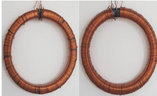
Figure 3. References magnetic circuits
