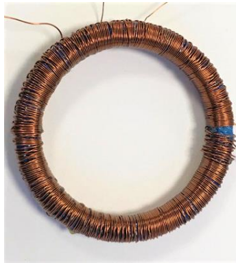
Figure 3 - Impregnated magnetic circuit with the non-porous adhesive tape
