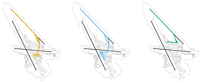
Figure 12. A subset of the clustered aircraft ground trajectories detected using positional features provided by ADS-B data.
