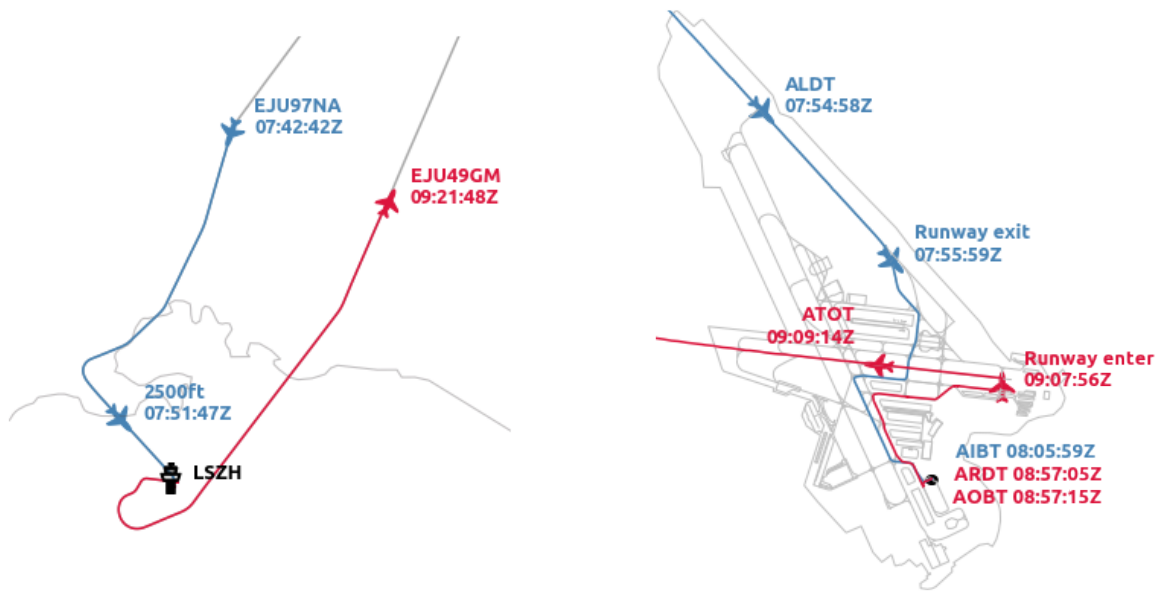
Figure 2. Tailored A-CDM milestones emphasizing airborne view (left) and airport surface view (right) of a sample aircraft movement. The arrival/ departure view shows aircraft enters the arrival sequencing and metering area (ASMA), is on final approach and leaves ASMA. On the surface, the aircraft passes the following milestones: actual landing time (ALDT), leaving runway at exit point, actual in/off-block time (AIBT, AOBT), aircraft ready time (ARDT), entering runway, actual take off time (ATOT).
