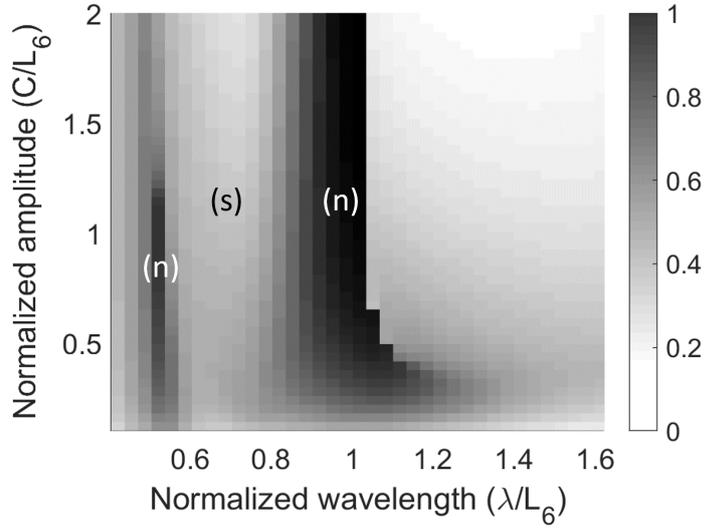
**Figure 14.** Mapping of the linearized transfer function for the bicycle, built with the vertical displacement amplitude that occurs at the excitation wavelength induced by the ground profile ( $C_F(\lambda_0, a)$ , equation (5)). The bicycle architecture behaves like an efficient filter except for wavelengths close to the spacing between wheels or its half (points (n)), for which a poor efficiency in the kinematic filtering is observed.
