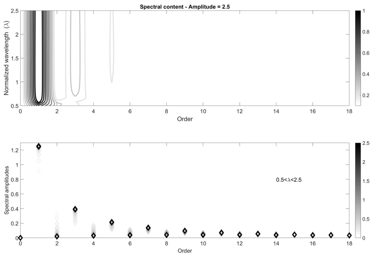
**Figure 18.** Spectral content versus wavelengths and amplitudes ( $S_v(1/\lambda)$  in equation (6)) for a single wheel: the natural kinematic filtering induces a nonlinear behavior with odd harmonics.
