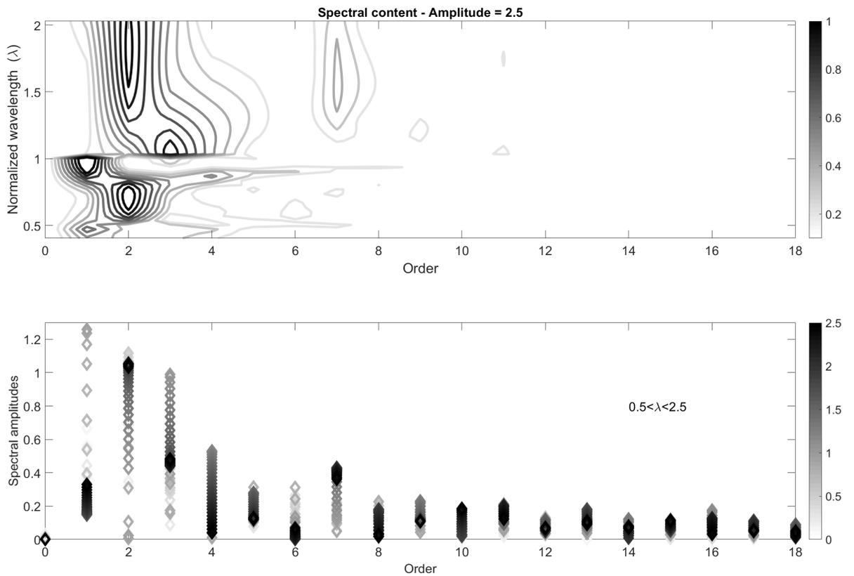
**Figure 19.** Spectral content versus wavelengths and amplitudes ( $S_v(1/\lambda)$  in equation (6)) for a double wheeled system (bicycle): the filtering effect combines the effect of a single wheel and the distance between wheels. The system is clearly efficient except for wavelengths equal to the distance between wheel and its half.
