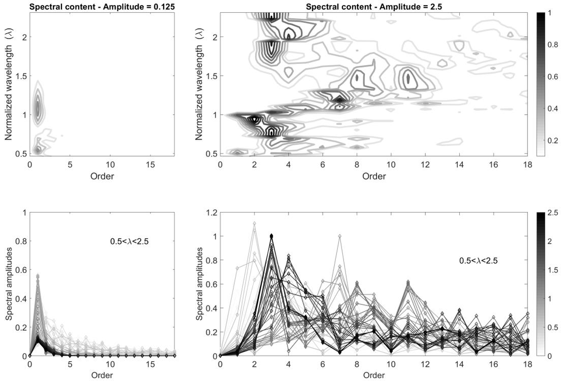
**Figure 20.** Spectral content versus wavelengths and amplitudes ( $S_v(1/\lambda)$  in equation (6)) for the rocker-bogie system: for small amplitudes (left part) the system acts as a linear system without harmonic content; when the amplitude increases (right part), nonlinearities introduce harmonics and the spectral energy goes to higher frequencies domain.
