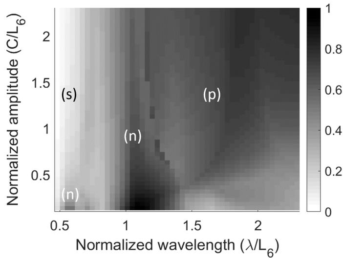
**Figure 13.** Mapping of the filtering effect of the rocker-bogie system based on the displacement amplitude criterion  $C(\lambda, a)$ , normalized to the distance between wheels. The filtering effect of the rocker-bogie architecture is globally better than that of the bicycle. Nonlinearities depending on high amplitudes are greater than those observed for the bicycle.
