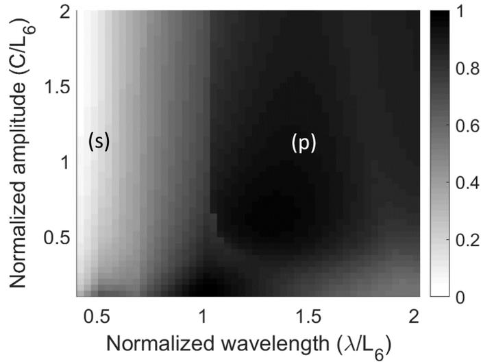
**Figure 12.** Mapping of the filtering effect of a bicycle based on the displacement amplitude criterion  $C(\lambda, a)$ , normalized to the distance between wheels. A good efficiency for wavelengths smaller than spacing between wheels is observed.
