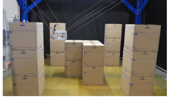
Fig. 10: CDPR prototype and cluttered environment made up of 18 boxes
