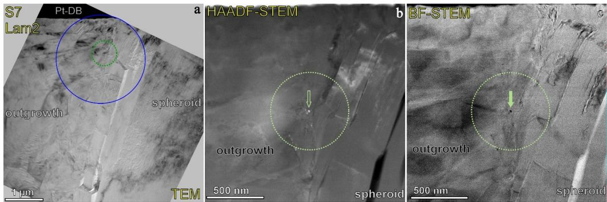
Fig. 9 TEM image (a), HAADF-STEM (b) and BF-STEM (c) images. The large solid circle corresponds to that in figure 7(a); dashed circles mark out the same sample area in the three images; the small arrows point to the small inclusion exhibiting a bright contrast on HAADF-STEM image (b) and a dark one on BF-STEM image (c).
