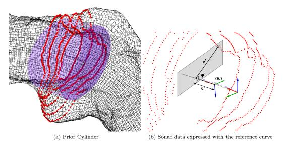
Figure 4: Modification of original method in [5] using a reference curve instead of the robot trajectory
