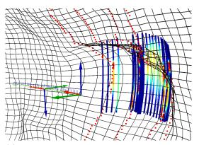
(b) Scaled-beta distribution of estimated elevation angles for horizontal sonar measurements from the first scan
