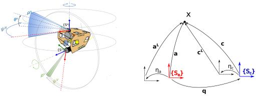
(a) Illustration of the robot mounted with two perpendicular sonar
