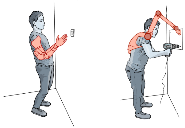
Fig. 1: Humans utilizing their kinematic redundancies to compensate for the lack of collaboration in wearable robots. In (a), the human leans backward to create an upward motion at the end-effector of the prosthetic arm, and in (b), leans forward to create forward motion at the end-effector of the supernumerary arm.
