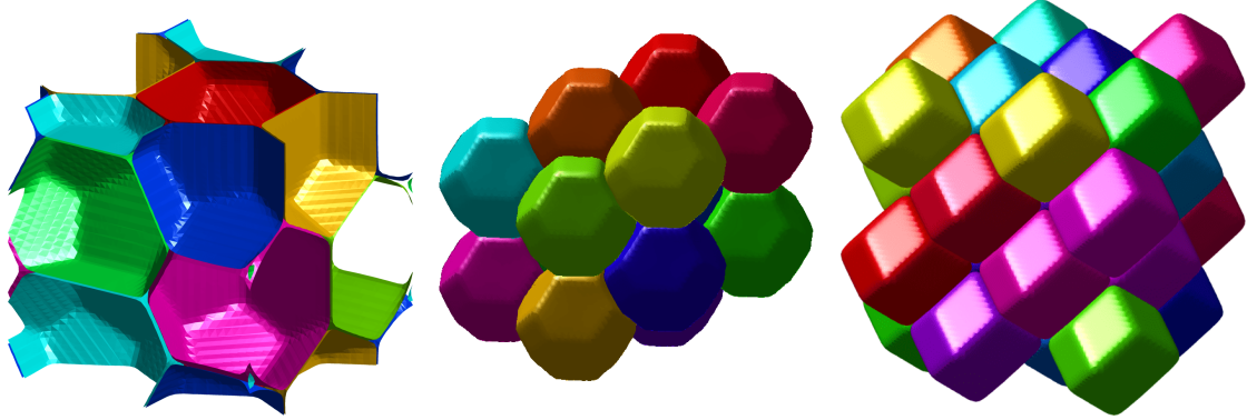
Figure 14: Some computations on the periodic cube: the Weaire-Phelan structure for n = 8 , the Kelvin structure for n = 16 and the rhombic dodecahedron structure for n = 32 .
