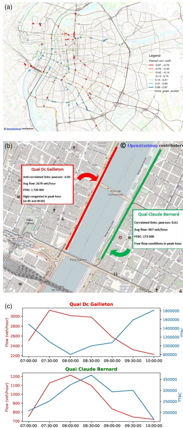
Fig 7. Per-edge temporal correlation between BC and flow (a) and zoom on a specific region (b,c). (a) Per-edge temporal correlation (only edges equipped with loop detectors have a non-null value) (b) Zoom on an area with two roads: Quai Dr. Gailleton and Quai Claude Bernard (c) Evolution of the TTBC and flow on the road: Quai Dr. Gailleton and Quai Claude Bernard.
