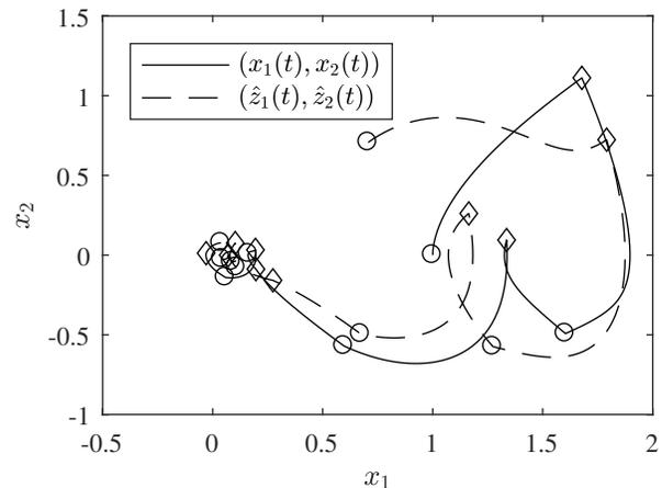
Fig. 1. Trajectory of the closed-loop system starting from  $x_0 = (1, 0)$  and  $\hat{z}_0 = (\sqrt{2}, \sqrt{2}, 1/2)$  over  $[0, 5T]$ , *i.e.*, after 5 switches from stabilization phase to observation phase ( $\circ$ ) and 5 switches from observation phase to stabilization phase ( $\diamond$ ).
